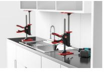
The optional installation kit BEY-IK provides even greater flexibility. This accessory set consists of an extension adapter and a rail unit. Quick, tool-free installation in combination with the BEYCEPS expands the usable area up to 620 mm, depending on the configuration, and supports up to 60 kg. This allows wall cabinets, floating sideboards or bathroom furniture, for example, to be mounted quickly and precisely.
